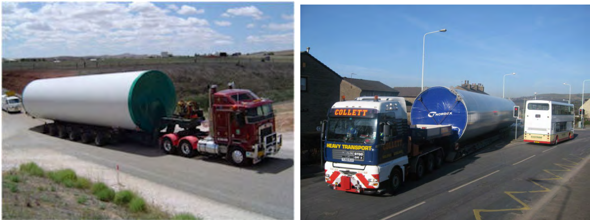
Figure 2-5: Transportation of a Tower section
